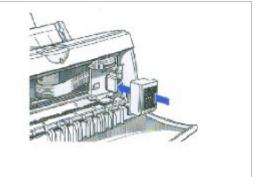
Press the lock lever down completely; do not use excessive force.
